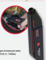
Angled nozzle fits to all types of motorcycle valves Measuring range 2–100 PSI (0.15–7.00 Bar) Accuracy +1% +0.5 PSI Power 3V Lithium battery
